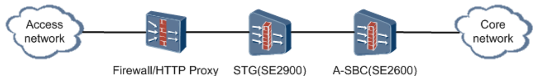
Figure 4-77 Networking with a standalone STG
