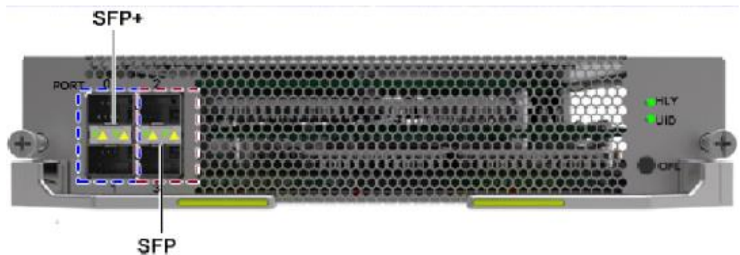
Figure 6-3 Ports on the VPUA0/VPUA1
