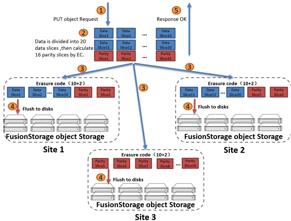
Figure 5-6 Data distribution of the three-site FusionStorage object storage cluster
