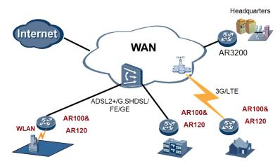
Example deployment in branch networks for WAN access. In this example, the AR100s and AR120s function as the egress routers on enterprise branch networks and provide multiple access methods, including Ethernet, xDSL, 3G, LTE and WLAN.
