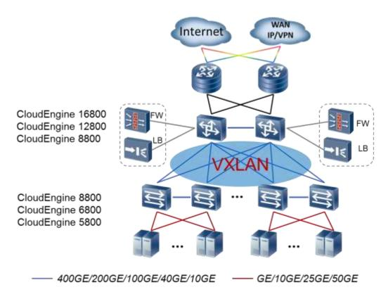
Note: VXLAN can also be used on campus networks to support flexible service deployment in different service areas.
