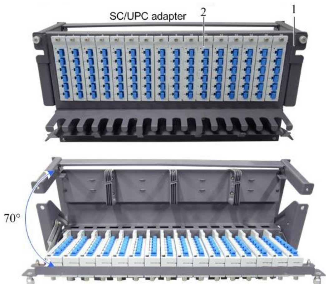
Figure 2-15 Appearance of the 5 U intermediate termination service processing subrack
