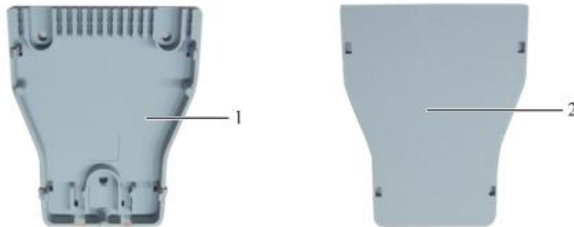
Figure 2-25 Appearance of the flat drop cable entry module
