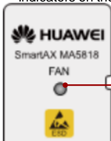
Indicators on the MA5818 fan tray
