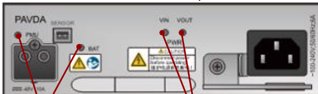
Indicators on the MA5818 power board
