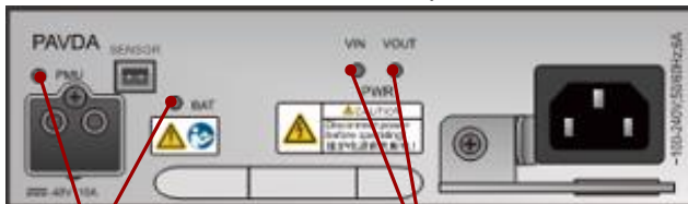
Indicators on the MA5818 power board
