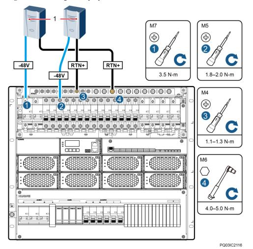
Figure 4-11 Installing DC output power cables
