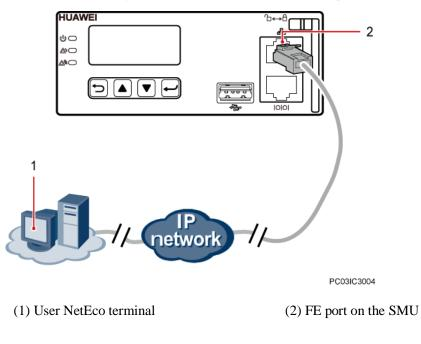
Figure 4-8 Connecting a communications cable (over the FE port)
