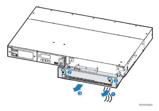
Step 4 Record the positions where the PCB connects to all the cables, and then disconnect the cables.Step 5 Remove the PCB.
