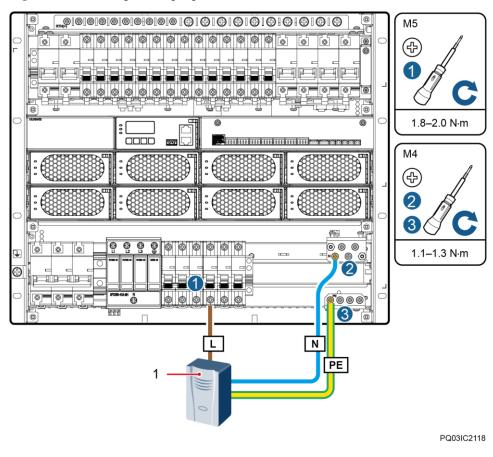
Figure 4-13 Installing AC output power cables
