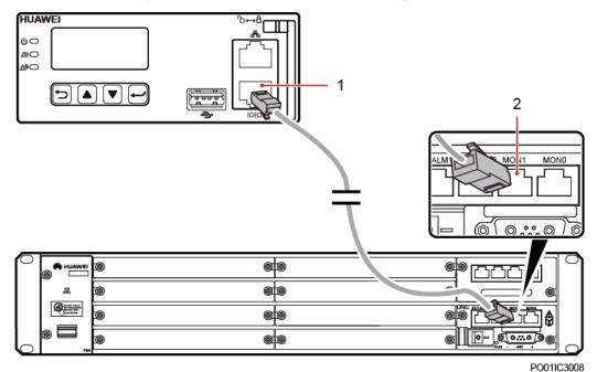
Figure 4-9 Connecting a communications cable (over the RS485 port)
