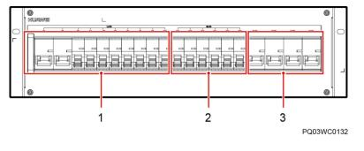
(1) LLVD circuit breakers (2) BLVD circuit breakers (3) Battery circuit breakers
