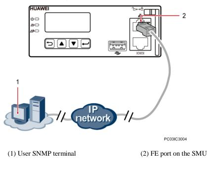
Figure 4-10 Connecting a communications cable (over SNMP)
