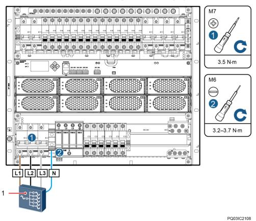
Figure 4-14 Installing 220/380 V AC three-phase, four-wire input power cables
