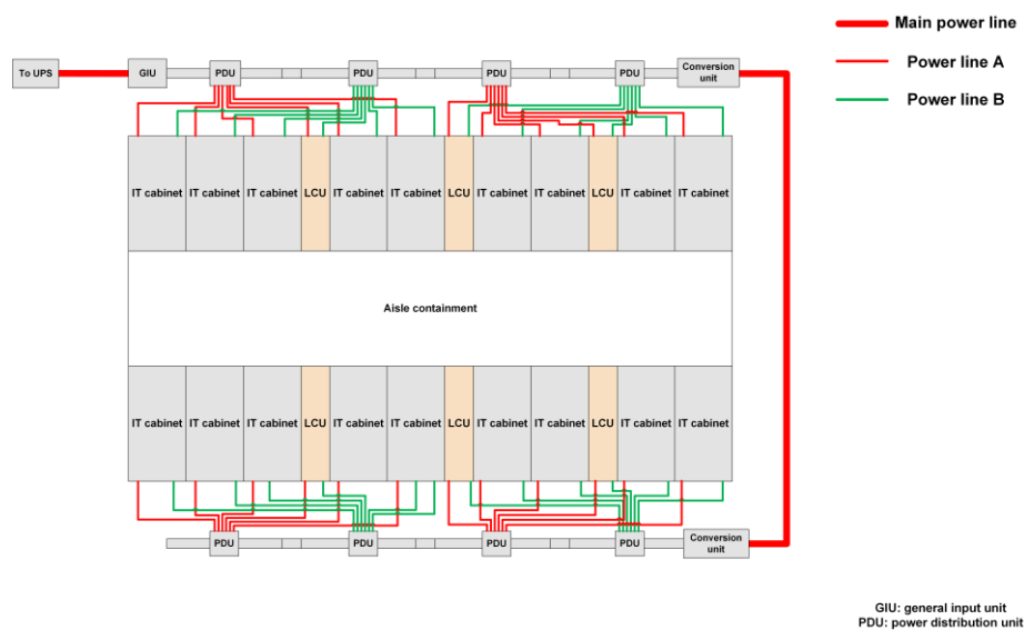
Figure 3-17 N+1 system power distribution diagram (new main way)
