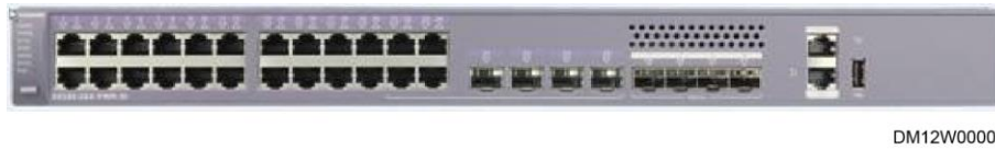
Figure 3-50 S5320 LAN switch
