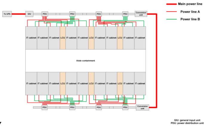
Figure 4-17 N+1 system power distribution diagram (new main way)
