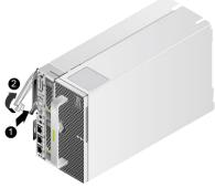
5. Insert the server node into the chassis horizontally until the server node cannot move forward, and lower the ejector lever. See steps (1) and (2) in the following figure.
