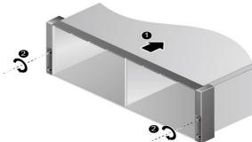
4. Press the latch on a server node and raise the ejector lever. See steps (1) and (2) in the following figure.
