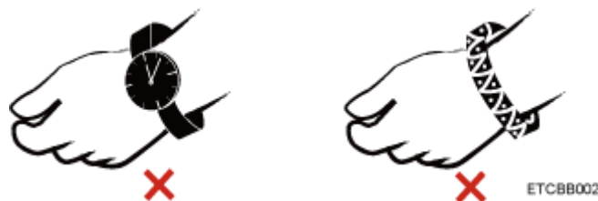
Figure 8-2 Conductive objects to be removed
