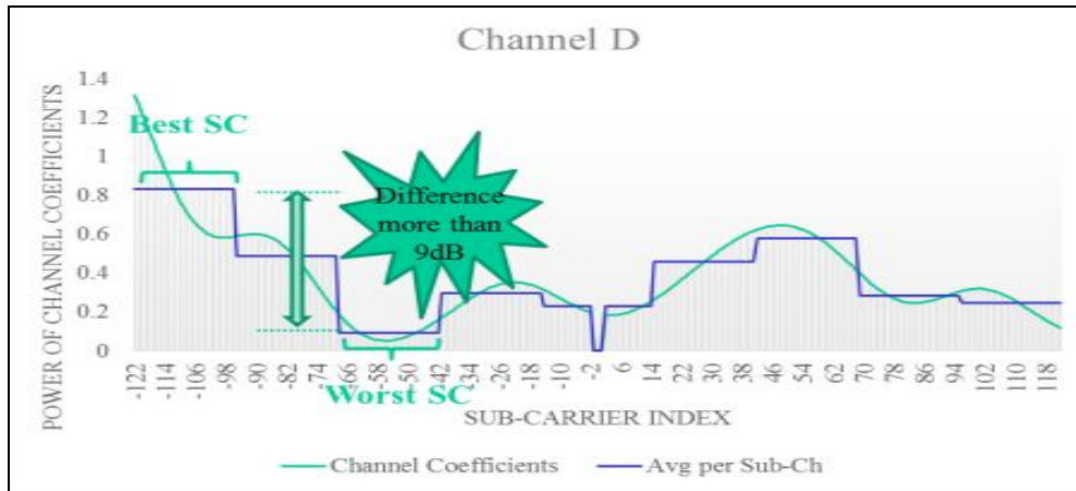
Figure 2-3 Channel quality in frequency domains of different subcarriers
