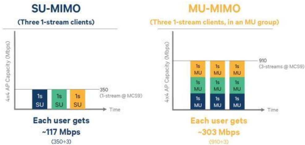
Figure 2-6 Throughput difference between SU-MIMO and MU-MIMO
