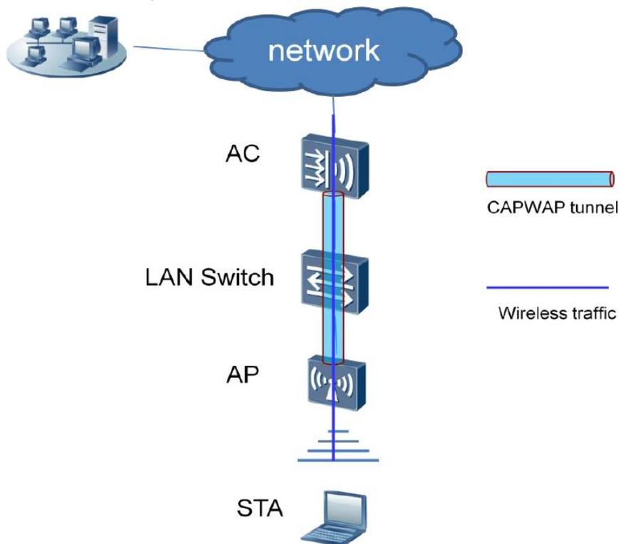
Huawei application identification function is supported only on WLAN ACs and applies only to the wireless user traffic transmitted in tunnel forwarding mode. To enable the application identification function in a Huawei WLAN system, the administrator needs to
