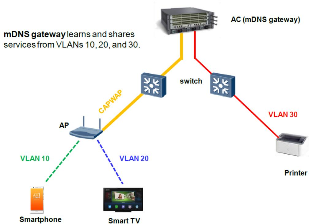
The WLAN AP uses the centralized forwarding mode, and forwards traffic from the smartphone and smart TV to the WLAN AC through the CAPWAP tunnel. The printer is also in the same VLAN as the WLAN AC. The switch between the printer and WLAN AC forwards traffic following the normal Layer 2 forwarding process. With the mDNS gateway function enabled, the WLAN AC maintains services in VLANs 10, 20, and 30, and responds to query requests, allowing service discovery across VLANs and network segments.
