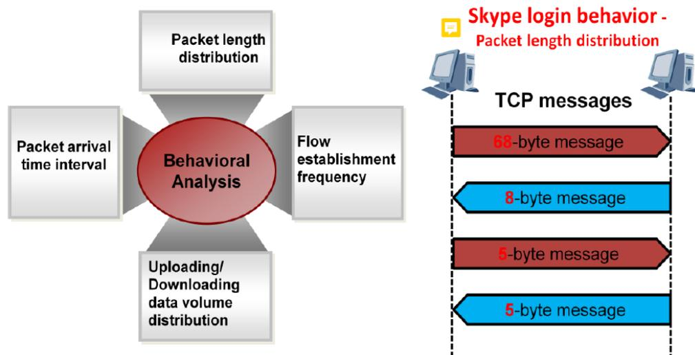
A small part of the Skype flows has signatures. TCP traffic sometimes uses ports 80 and 443, and UDP traffic sometimes uses ports 12340 and 12350, so a combination of port-based, signature-based, and behavior analysis-based identification methods can be used to identify the Skype traffic effectively.
