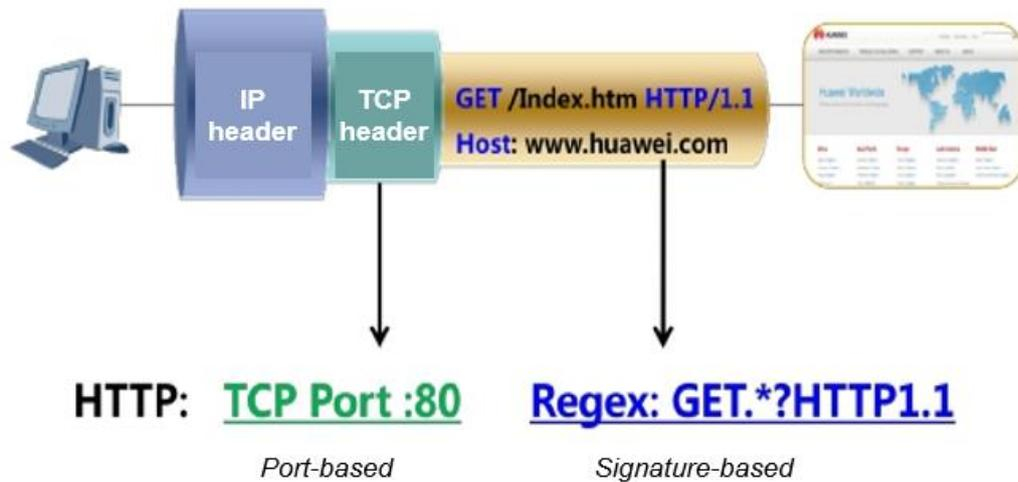
More than one identification methods are often used together to increase the identification accuracy. For example, HTTP identification based only on port numbers is inaccurate because port 80 can also be used by other applications. Therefore, signature-based identification method can be added to increase the identification accuracy.
