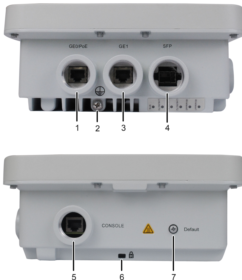
Figure 3-34 Interfaces on the AP
