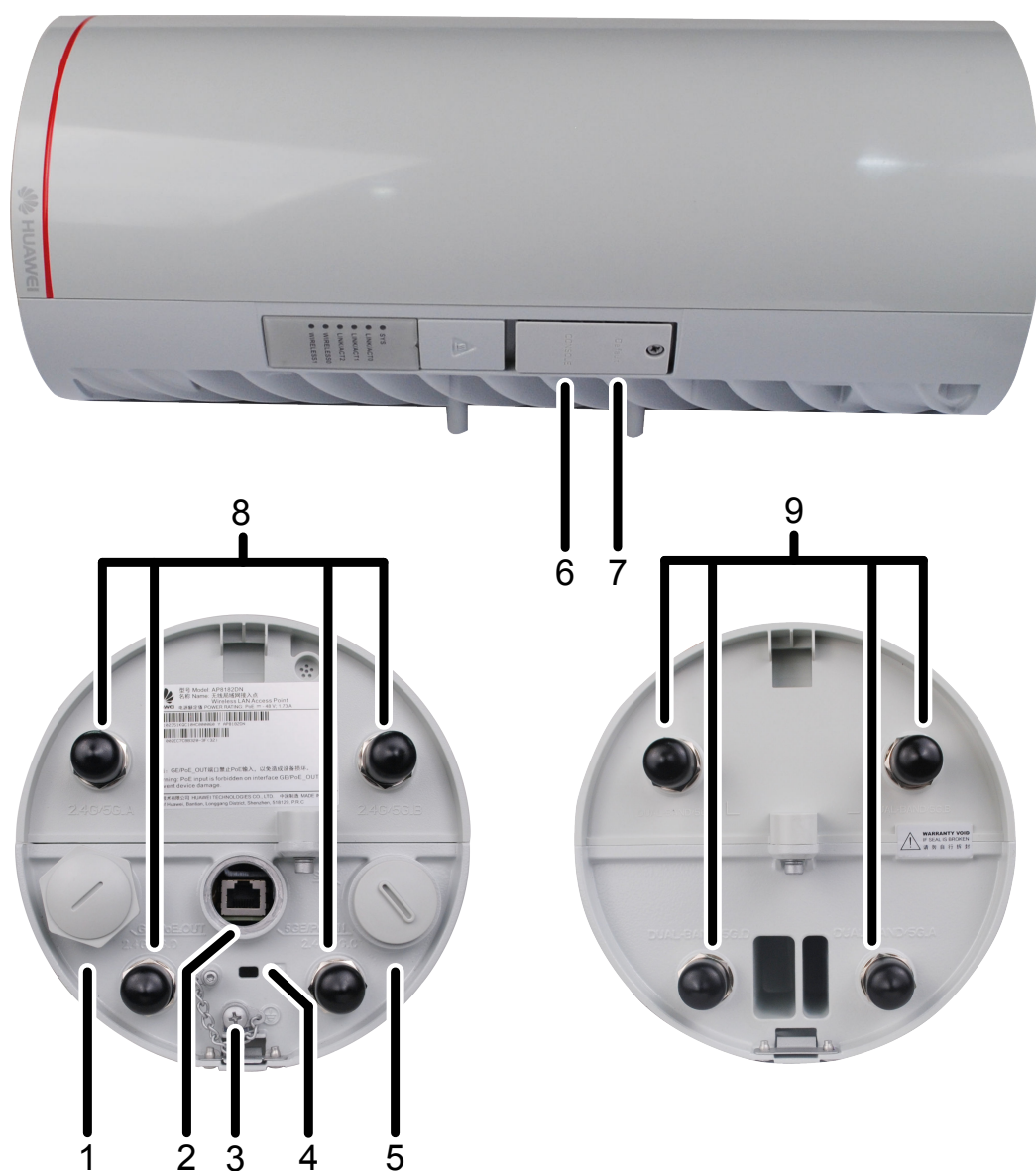
Figure 3-52 Interfaces on the AP
