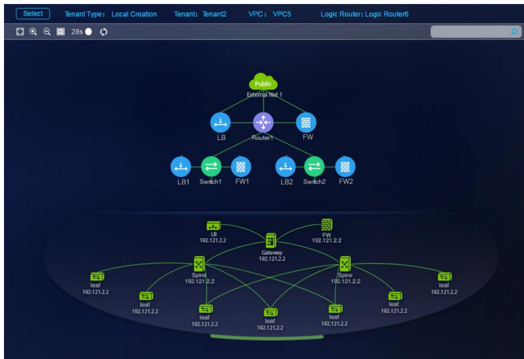
Figure 2-21 Mapping from the logical topology to the physical topology
