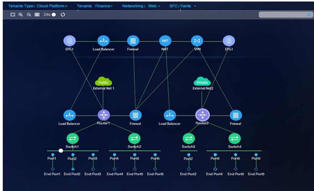
Figure 2-20 Mapping from the application topology to the logical topology
