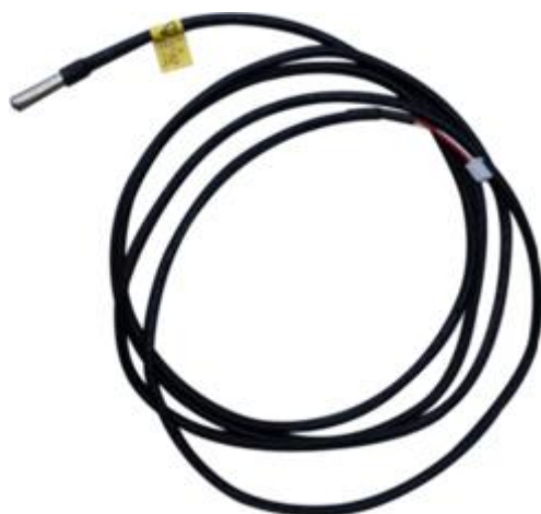
Figure 6-7 Appearance of the battery temperature sensor (NTC type)
