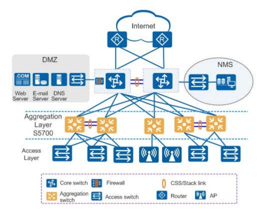
On an enterprise network or campus network, the CloudEngine S5731S-S switches connect to access switches through gigabit or 10 gigabit interfaces, provide high performance and large switching capacity, and connect to core switches through 10 gigabit optical interfaces. The network provides 10 Gbit/s rate for the backbone layer and 100 Mbit/s access rate for terminals, meeting requirements for high bandwidth and multi-service.
