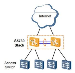
Other than that, the CloudEngine S5731S-S switches can be used as the core switches of a small-sized enterprise campus network, which have powerful aggregation and routing capabilities. The CloudEngine S5731S-S switches use iStack to ensure high reliability. The switches provide various access control policies to achieve centralized user management and simplify configuration.
