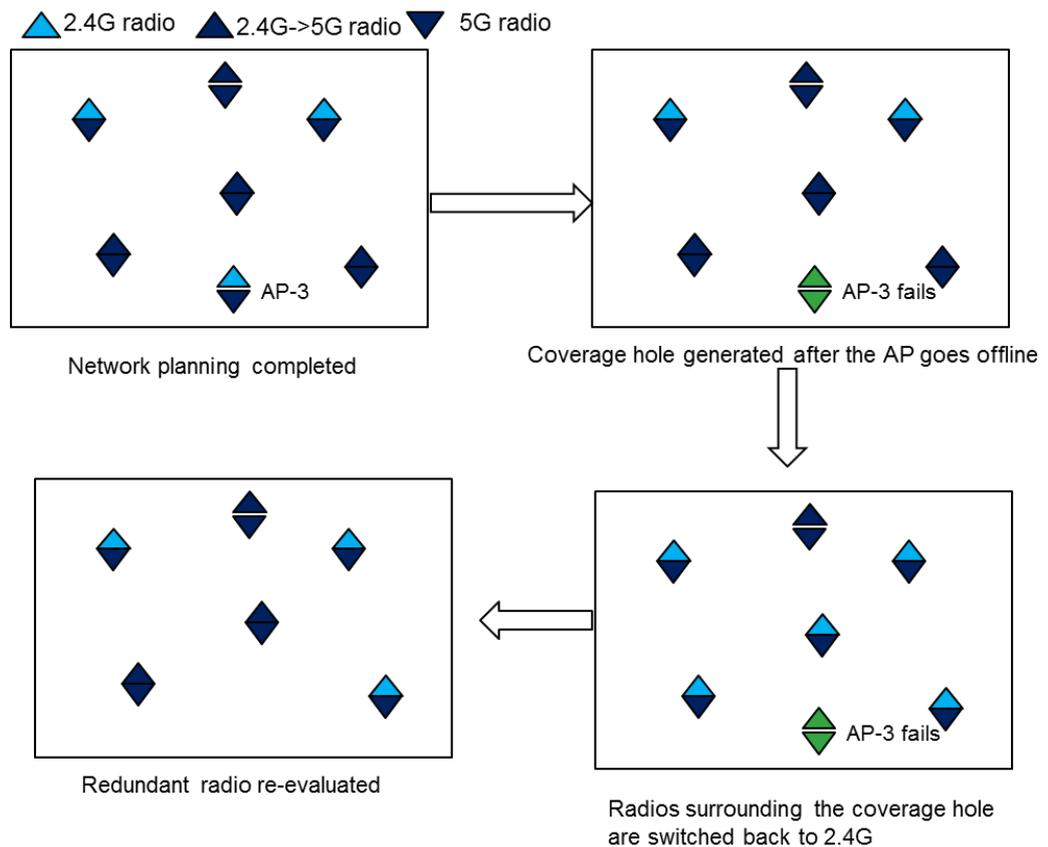
As shown in the preceding figure, AP3 becomes faulty, and Wi-Fi signals disappear. The system performs the following operations to address this issue:
