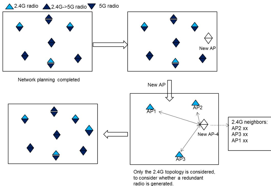
1. Scan and add APs to construct a 2.4 GHz topology.
