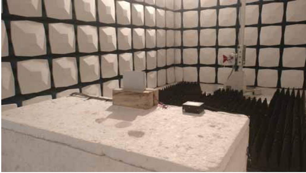
Figure 6 Radiated Emission test setup (Above 1GHz)
