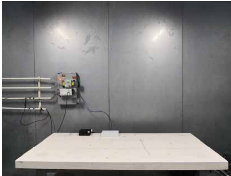
Figure 4 Conducted Emission test setup
