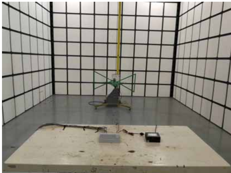
Figure 5 Radiated Emission test setup (Below 1GHz)
