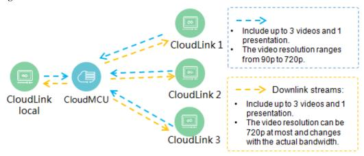
For example, five SVC participants join a conference and a participant is sharing the presentation. Each participant's terminal can send multiple streams to the CloudMCU for forwarding. Based on the local continuous presence mode, the local soft client can receive streams of different resolutions from other participants. **Figure 3-11** shows the local video modes and corresponding resolutions.
