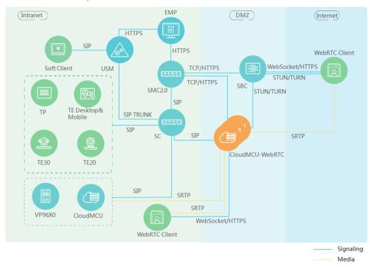
**Figure 3-6** Deploying CloudMCU-WebRTC Gateway in the DMZ (SBC Functioning as the STUN/TURN Server)
