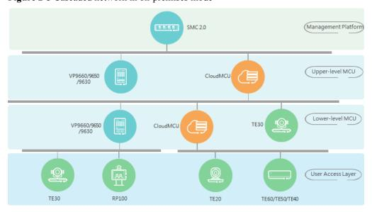
Figure 2-5 Cascaded network in on-premises mode
