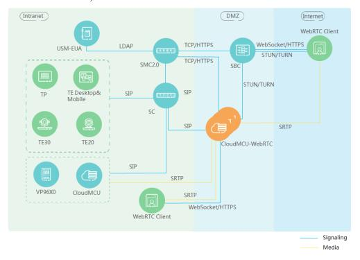
The CloudMCU, which works as the WebRTC gateway, is deployed in the DMZ. Using the CloudMCU, the WebRTC client on the public network connects to Huawei videoconferencing system through web pages.
