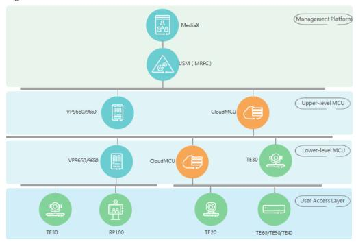
Figure 2-6 Cascaded network in hosted mode
