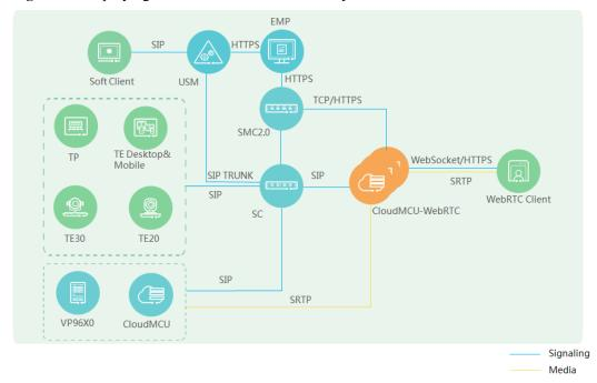
Figure 3-4 Deploying CloudMCU-WebRTC Gateway in the Intranet
