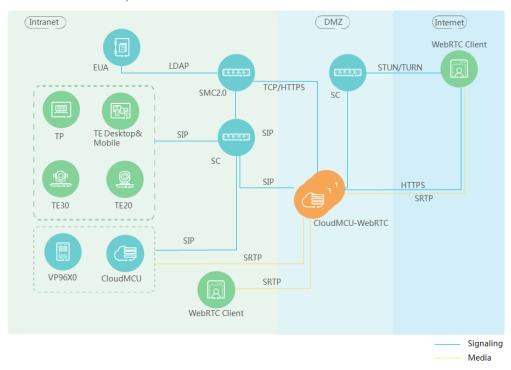
**Figure 3-8** Deploying CloudMCU-WebRTC Gateway in the DMZ (SC Functioning as the STUN/TURN Server)
