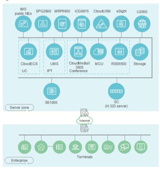
On an IMS hosted network, the IMS Core, MediaX, MCU (VP9600 series MCU or CloudMCU), USM, eSight, SBC, U2000, RSE6500, videoconferencing endpoints, and IP network are deployed. The MCU functions as the media switching platform in the system.
