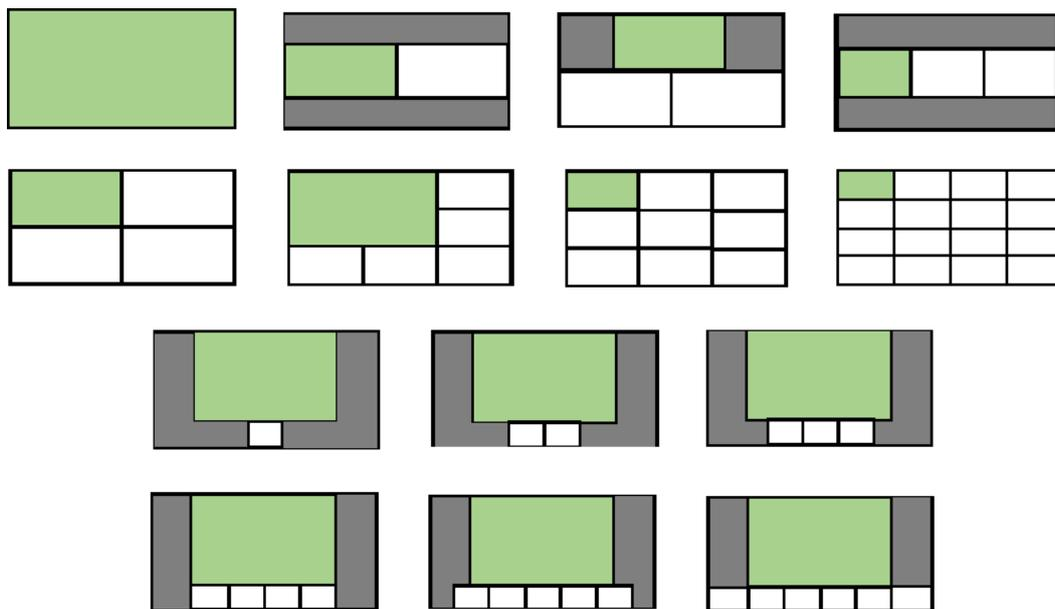
**Figure 3-3** Automatic continuous presence layouts
