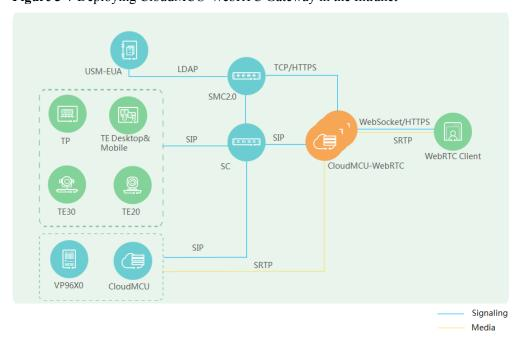
Figure 3-7 Deploying CloudMCU-WebRTC Gateway in the Intranet
