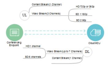
Fixed HD and SD modes are supported from the CloudMCU to SVC conferencing endpoints: 720p HD + 180p SD, or 360p HD + 90p SD. The detailed mode will be determined during signaling negotiation for joining conferences.
