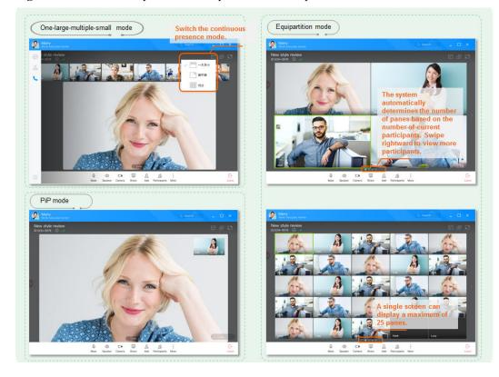
Figure 3-13 Continuous presence example on the desktop terminal
