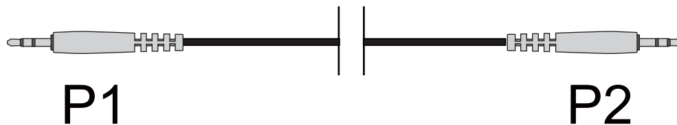
Figure 6-59 Structure of a 3.5 mm headset cable
