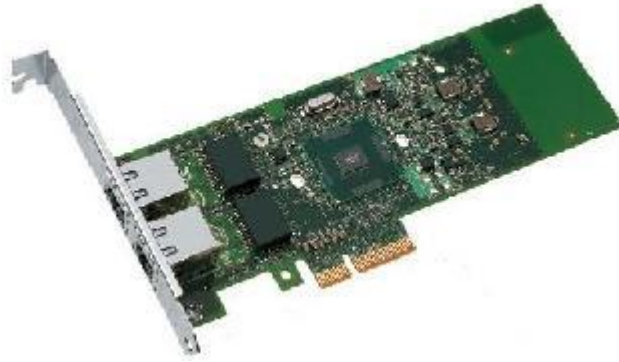
RJ45 Electrical Interface NIC
