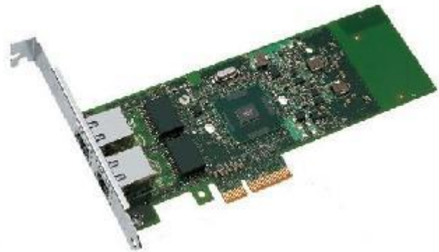
RJ45 Electrical Interface NIC
