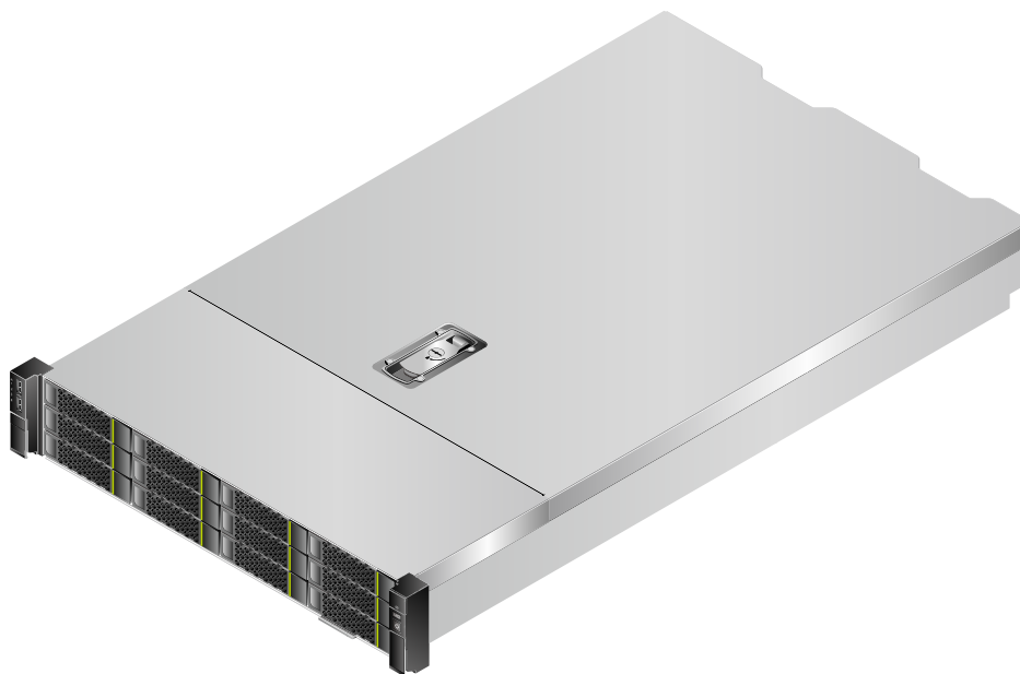
Figure 9-28 2288H V5 16-slot node overall appearance
