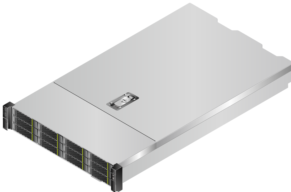
Figure 9-23 2288H V5 12-slot node overall appearance
