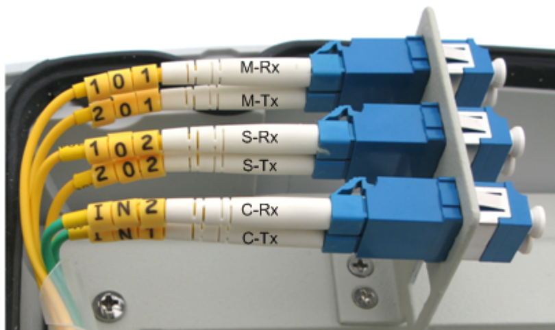
Figure 7-5 Fiber connection relationships
