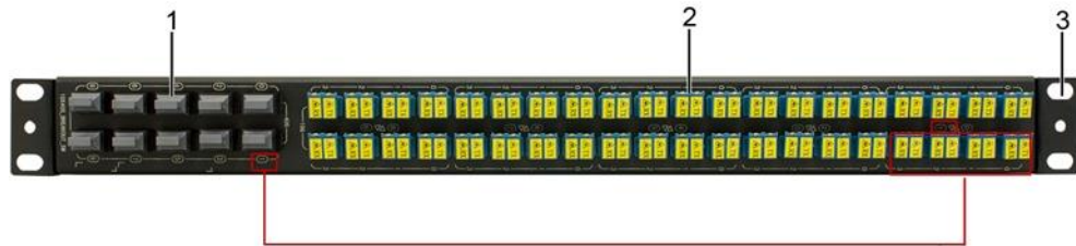
Figure 12-8 Mapping between MPO and LC adapters
