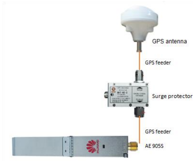
Figure 10-28 Connections between the AE 905S module, surge protector, and antenna
