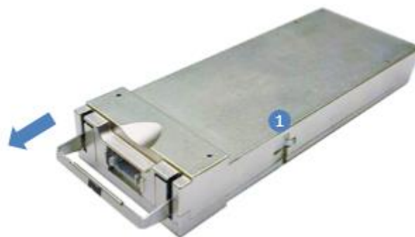
Figure 10-3 Removing a CFP2 optical module
