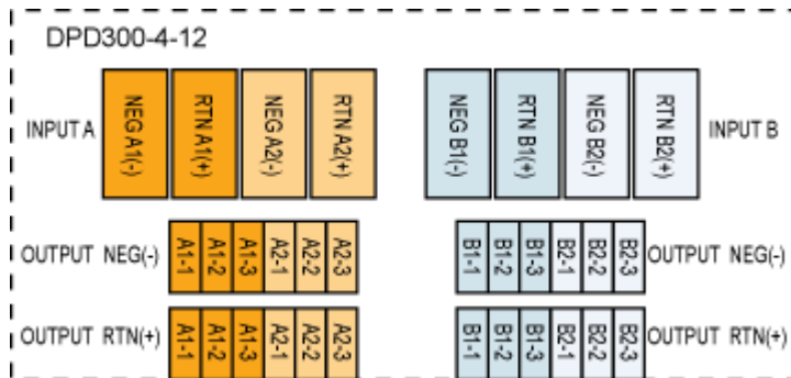
Figure 11-4 Mapping between input lines and output lines in the power distribution box
