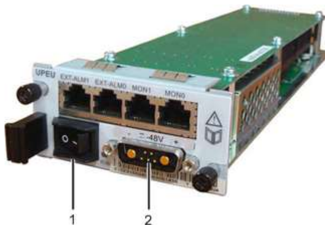
Figure 2-6 DC power supply module of the IAD1224
