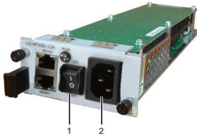
Figure 2-5 AC power supply module of the IAD1224
