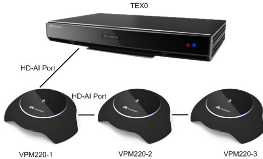
Figure 2-3 Network with multiple VPM220s
