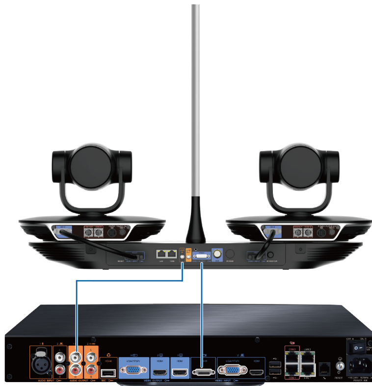
Figure 3-2 Connecting a VPT300 to a TE40 using the HD-VI cable
