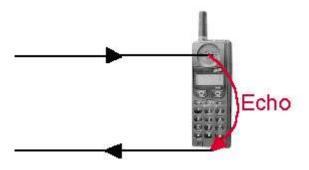
As shown in Figure 9-2, acoustic echo is generated when the voice from the handset is returned to the handset. The echo is more obvious during calls in speaker mode.
