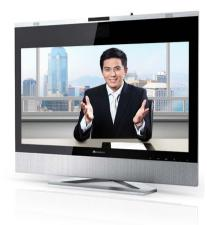
Huawei DP300 is a high-end, High Definition (HD) videoconferencing desktop endpoint. The system comes fully-integrated with an impressive HD (1080p 60fps) digital camera, High Fidelity (Hi-Fi) speakers, HD microphone, and 27-inch touch screen. The fashionable, sleek design provides you with an unprecedented audiovisual experience.
