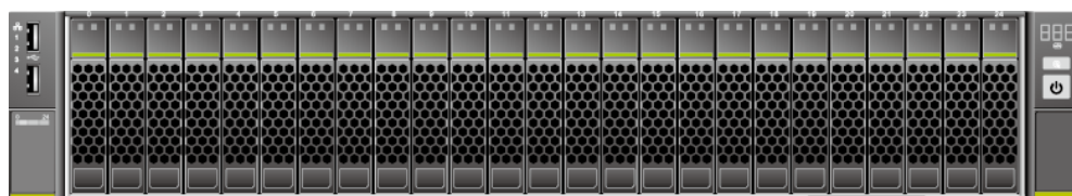
Figure 4-2 Front panel of the 2488 V5 with 25 SAS/SATA drives
