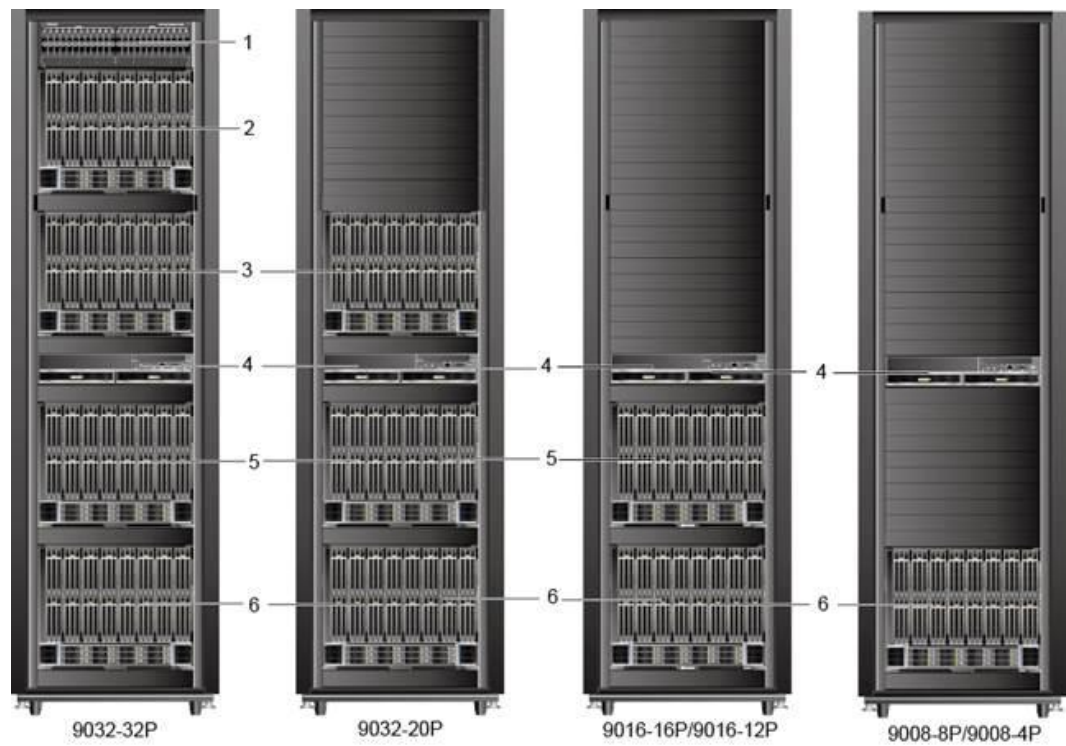
Figure 1-2 Front views of the 9032, 9016, and 9008 (single cabinet, without REEs)
