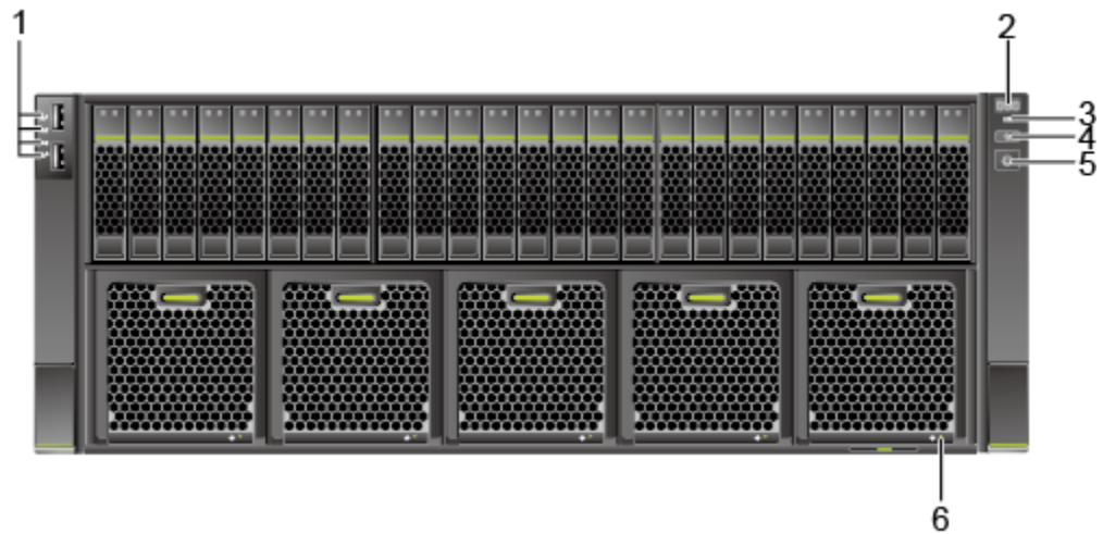
Figure 4-15 Indicators and buttons on the front panel of a server with 25 SAS/SATA drives
