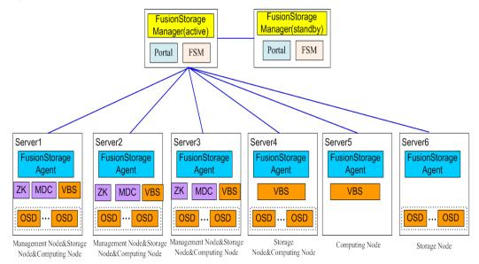
Figure 3-3 Logical architecture of FusionStorage Block
