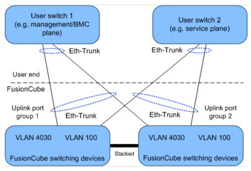
Figure 3-42 Uplink interconnection when management and service planes are physically isolated
