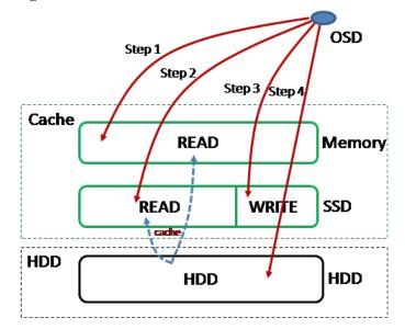
Figure 3-6 Read cache mechanism
