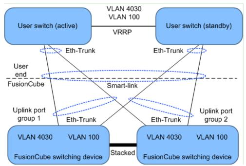
• User switches or routers work in active/standby mode using VRRP. An independent VLAN is used to control VRRP heartbeats on the switches. User switches and the FusionCube switching devices support Eth-Trunk (or port aggregation).
