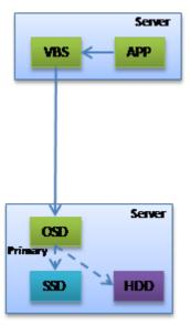
An application delivers a read I/O request to the OS. The OS forwards the read I/O request to the VBS of the local server. The VBS uses the data routing mechanism (for details, see **3.2.2.1 Data Routing**) to identify the primary OSD where the data is located based on the LUN and LBA information in the read I/O request. If the primary OSD is faulty, the VBS reads the data from the secondary OSD.
