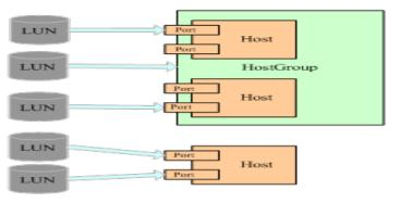
Figure 3-11 Mapping between LUN Masking components
