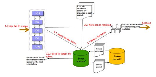
The token bucket C is used for I/O control. The token bucket E is used to store the remaining tokens. The two buckets work together to implement the burst function.
