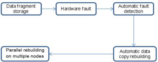
FusionStorage Block supports parallel and rapid data rebuild as follows:
