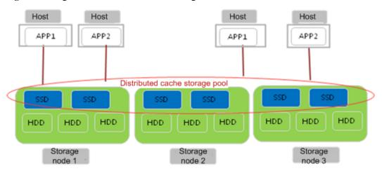
Figure 4-2 Logical architecture of FusionStorage Block distributed cache
