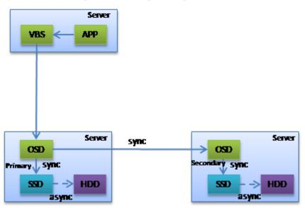
Figure 3-8 Write I/O process (two-copy backup)
