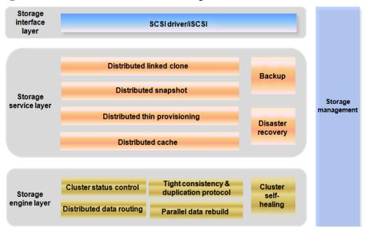
Figure 3-2 Functional architecture of FusionStorage Block
