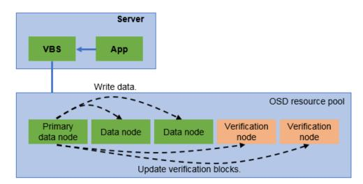
An application delivers a write I/O request to the OS. The OS forwards the I/O request to the VBS of the local server. The VBS uses the data routing mechanism to determine the primary OSD where the data is located based on the LUN and LBA information in the write I/O request.
