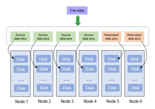
Example: Four source data slices and two redundant data slices are stored on six nodes.
