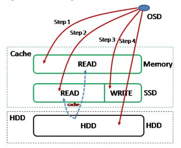
Figure 4-4 FusionStorage Block read cache mechanism
