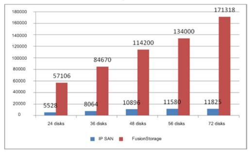
Figure 4-6 FusionStorage and IP SAN comparison test
