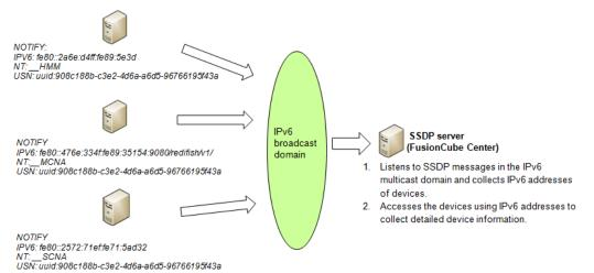
The process of automatic device discover during system installation is as follows:
