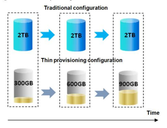
Figure 3-12 Automatic thin provisioning mechanism
