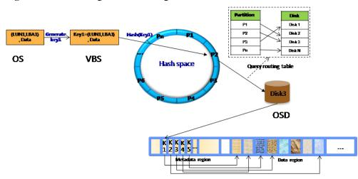
Figure 3-4 Data routing of FusionStorage Block
