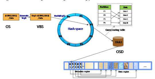
Figure 4-1 FusionStorage block storage data routing process
