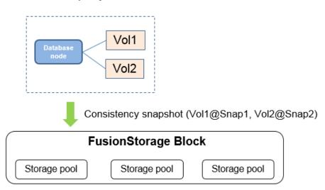
Figure 3-14 Consistency snapshot mechanism
