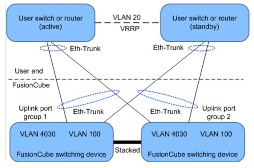
**Figure 3-44** Uplink interconnection using an independent VLAN for VRRP heartbeat control when management and service planes are converged
