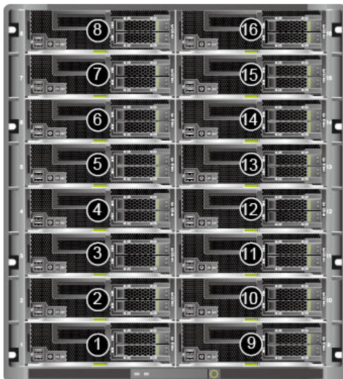
Figure 1-2 Installation positions and slot numbering
