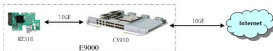
Figure 3-3 Connection between the MZ310 and the CX910
