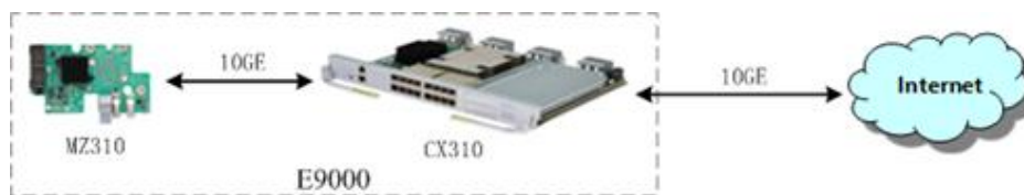
Figure 3-2 Connection between the MZ310 and the CX310
