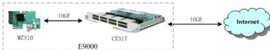
Figure 3-4 Connection between the MZ310 and the CX317
