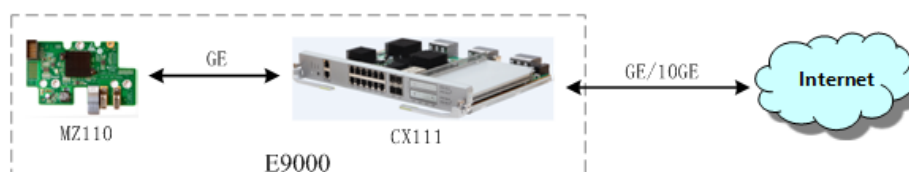
Figure 3-3 Connection between the MZ110 and the CX111
