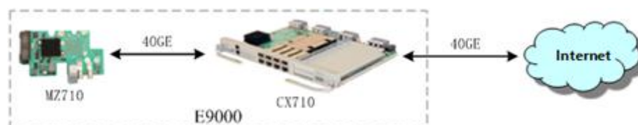
Figure 3-2 Connection between the MZ710 and the CX710
