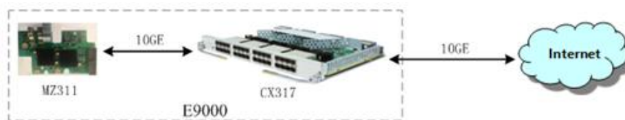
Figure 3-4 Connection between the MZ311 and the CX317
