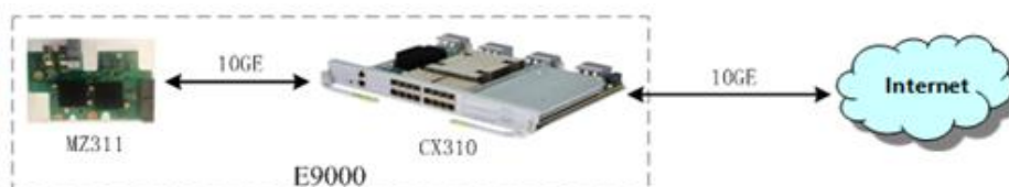
Figure 3-2 Connection between the MZ311 and the CX310
