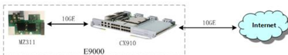
Figure 3-3 Connection between the MZ311 and the CX910
