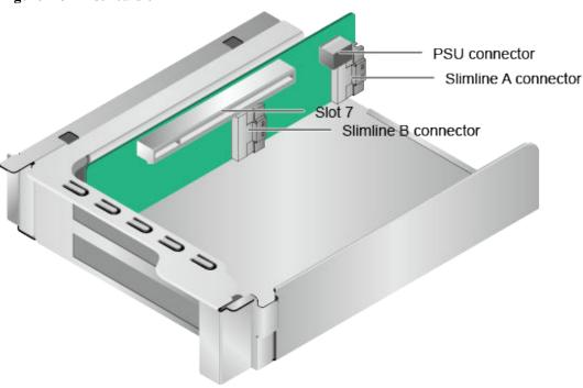
Figure 4-35 shows the PCIe slots on the rear panel.
