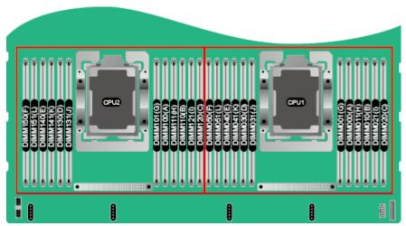
• The server supports DIMMs of 8, 16, 32, 64, and 128 GB. A server fully configured with DIMMs provides up to 3072 GB memory.
