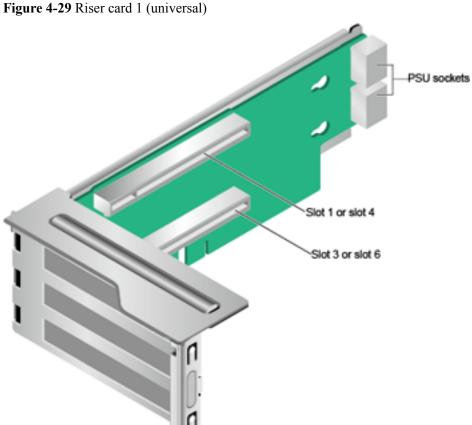
When installed in I/O module 1, this riser card provides slots 1 and 3. When installed in I/O module 2, this riser card provides slots 4 and 6.
