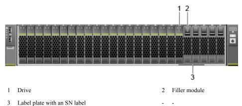
• **Figure 4-4** shows the front panel of a server with twenty-four 2.5-inch drives.
