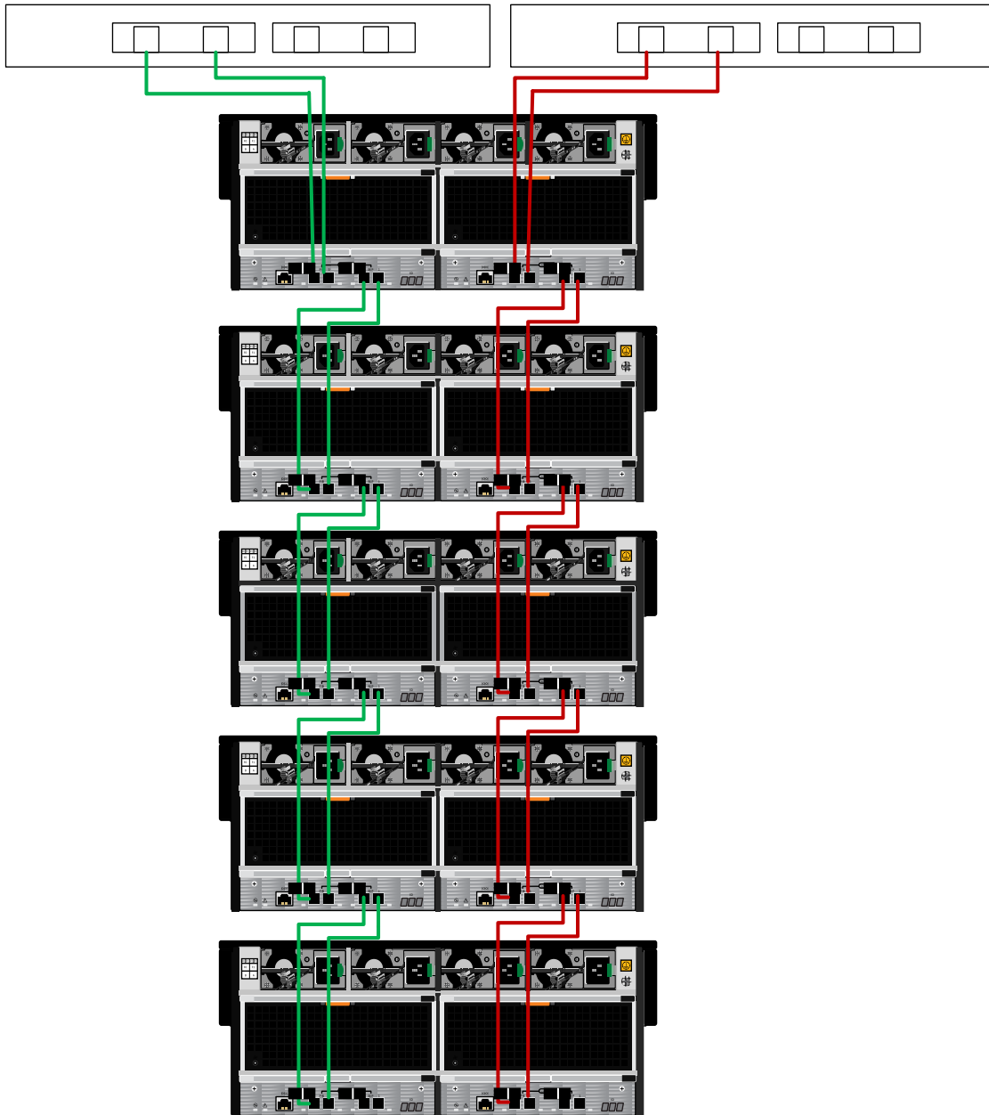
Figure 4-9 Dual-link redundant networking in forward connections
