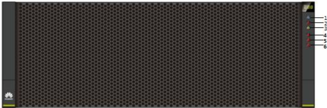
Figure 3-9 High-density disk enclosure front-panel indicators
