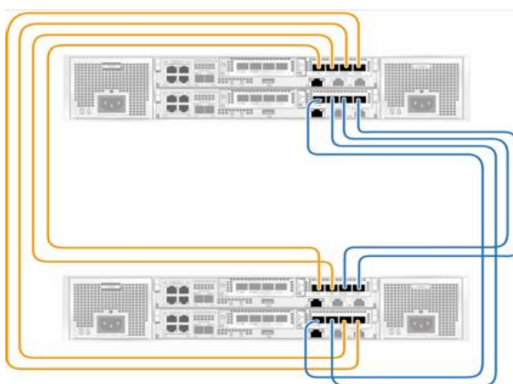
Figure 3-3 Direct-connection network employing a four-controller architecture
