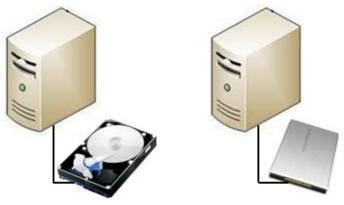
In the previous figure, the left drive is an HDD and its IOPS is calculated as follows: 1/5 ms = 200 IOPS
