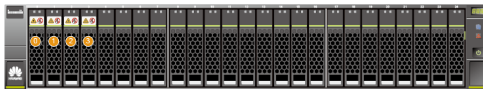
Figure 4-58 Positions of external coffer disks in the disk and controller integration architecture
