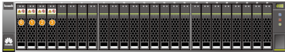
Figure 4-113 Positions of external coffer disks in the disk and controller separation architecture
