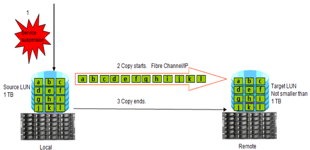
Figure 5-11 HyperCopy working principle
