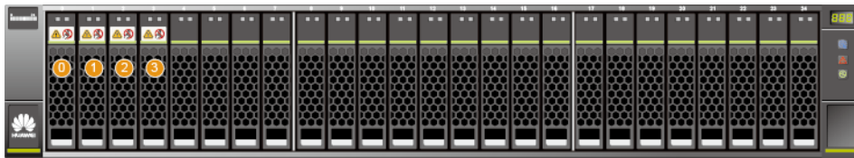
Figure 4-38 Positions of external coffer disks
