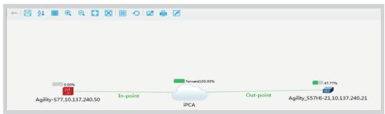
Path hop-by-hop detection can locate the node or link where packets are lost in an area.
