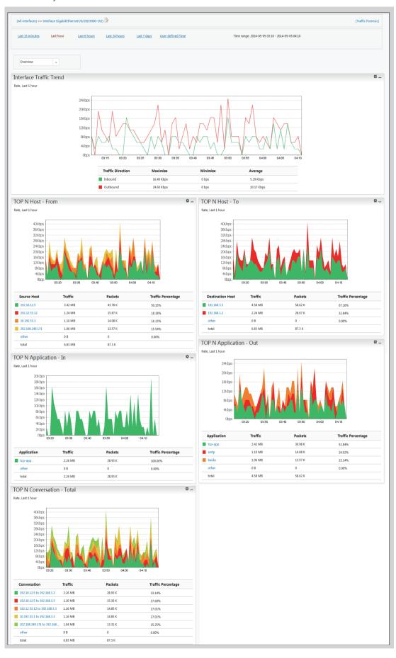
Interface traffic analysis checks the traffic trend for a specified interface, time range, and incoming and outgoing traffic. Based on interface traffic analysis, network administrators can identify the interfaces that are used most frequently on the network to gain a comprehensive understanding of the entire network status. Administrators can detect interfaces with abnormal traffic and locate faults before network performance is affected.
