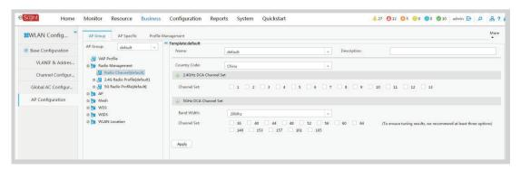
• Various VAP and radio profiles are preset and can be used repeatedly to improve the configuration efficiency. Parameters in the profiles are set based on administrators' experience, facilitating similar configurations by other administrators.
