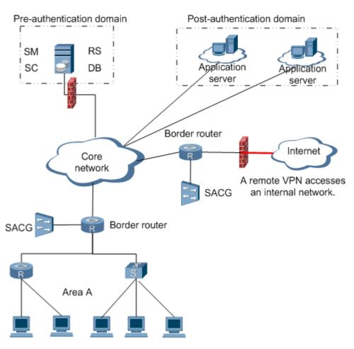
In this networking mode, the Agile Controller servers, including the SM server, SC server, RS server, and database server, are deployed in the same security zone. A firewall must be configured on the incoming path of the Agile Controller servers and firewall policies need to be configured based on the communication matrix of the system to prevent malicious attacks by terminals.
