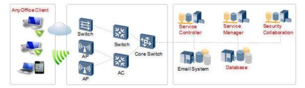
The Agile Controller can be deployed in a centralized or distributed manner. You can deploy the SM and SC on the same server, or deploy multiple SC servers separately.
