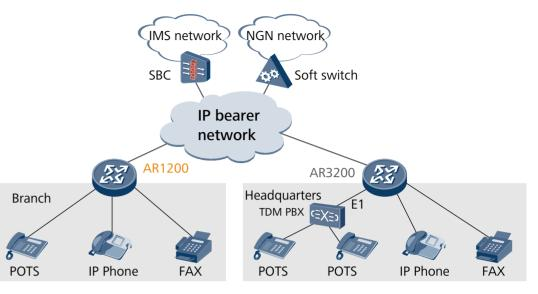
The AR1200 integrates voice, fax, and IP services. For enterprise users, the AR1200 serves as the SIP access gateway for a branch office, transforming phone signals into VoIP signals. The AR1200 uplink interfaces connect to the IP Multimedia Subsystem (IMS) or Next Generation Network (NGN) to allow any media, including phones, handsets, and computers, to communicate at any time.
