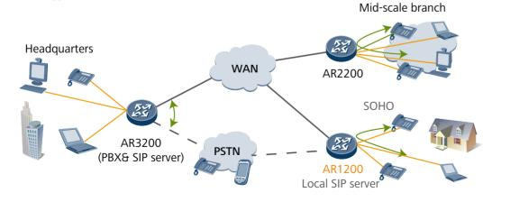
To enhance the corporate image and improve communication efficiency, all AR routers include a built-in PBX. This feature supports the enterprise main number, Interactive Voice Response (IVR), and bill query functions. The AR1200 can also be located in a branch office to provide intelligent dialing.
